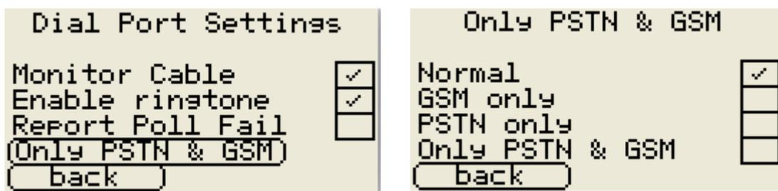
**Normal** – After an inter-digit timeout, if the called number is prefixed with '9' it will be routed over PSTN if PSTN is connected, otherwise it will be routed over GSM. If the called number is prefixed '7' will be routed over GSM straight away.
