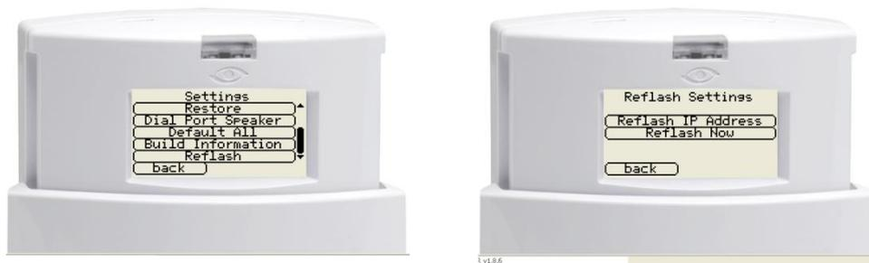
The reflash IP address is set by default to Chiron's reflash server (80.176.196.134) and does not need to be changed unless another reflash server is to be used. Please also note that a new IP address (195.59.117.164) has also been made available for the same reflash server giving access via a high speed fibre line. Improved performance can be expected if this new address is used.
