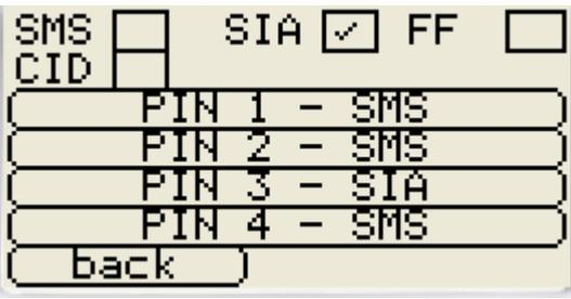
It is now possible to have a set up with alarms and SMS messages on different inputs.
