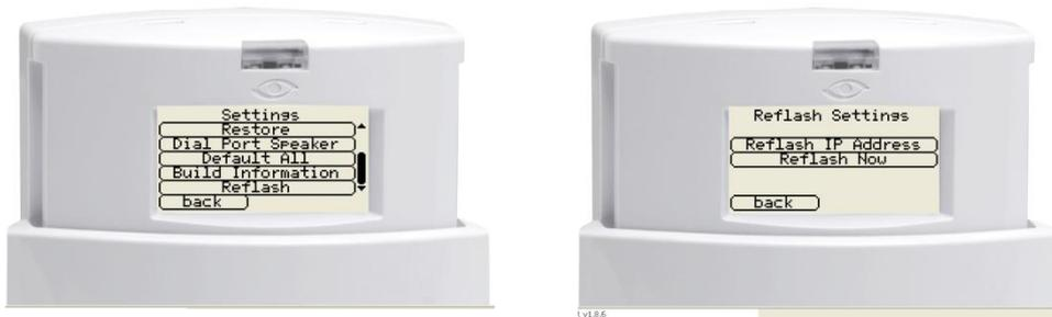
The reflash IP address is set by default to Chiron's reflash server (195.59.117.164) and does not need to be changed unless another reflash server is to be used.
