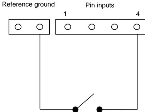
Opening the contact (i.e. loop is open circuit) generates an alarm signal.
