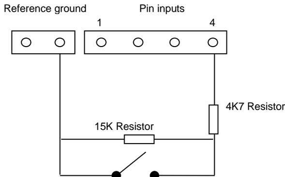
**Note:** For this feature to work correctly it is essential that the resistors are connected at the contact end of the loop and not the dialler end **and** that this monitoring is enabled on the dialler, which can either be done in the **Installation Wizard** for all inputs in use, or for each input individually in the **Settings** menu. The monitoring centre must also enable the monitoring of this facility on the dialler within the IRIS receiving system.
